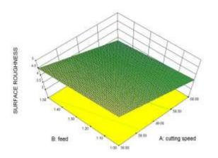
If cutting speed and feed increases the surface roughness will be low at high depth of cut.
